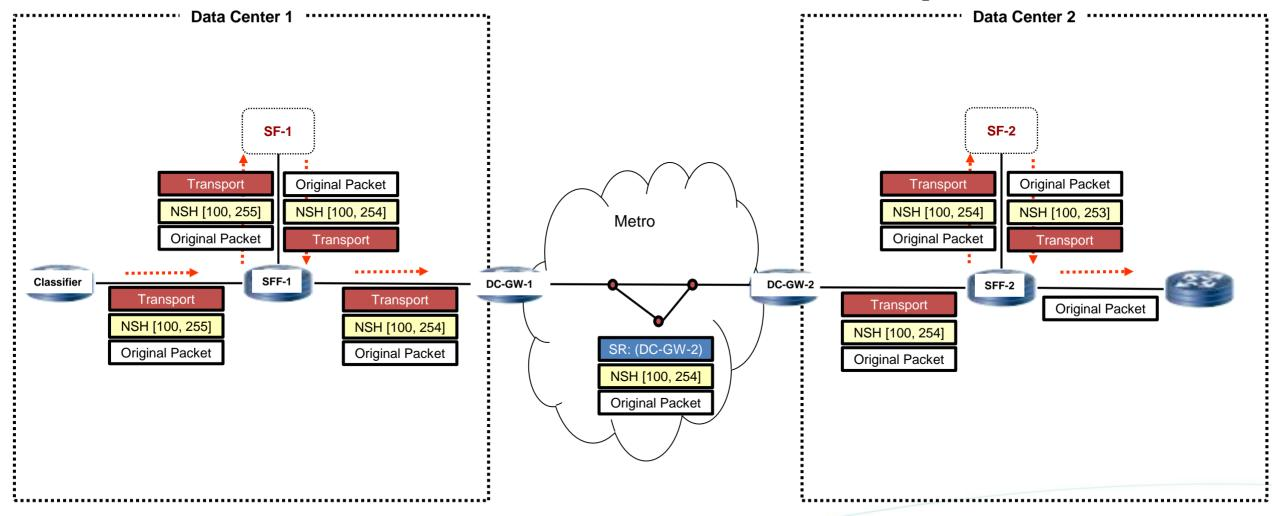
Totally decouple service & transport layers; leverage SR for traffic steering capabilities
